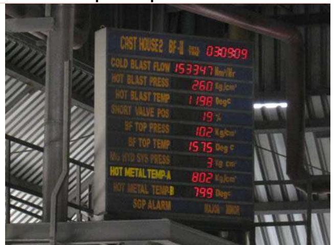
Blast furnace operation parameters
